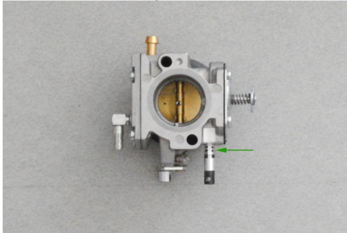
Whenever you choose to verify the carburetor settings, proceed in this way: completely close the screw L and H and then open them exactly with the standard setting, as described on chart 4.5. Remember: a strong pressure (tightening) on these screws can irretrievably damage the carburetor.
