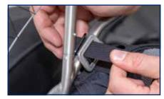
2) Remove both harness straps at the top of the airframe. Pay attention to how they are laced through the buckle
