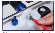
**9)** Secure the extended range tank in place using the M8 bolts previously removed. Tighten both bolts to 20Nm
