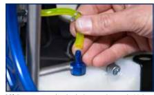
**10)** Reconnect the fuel pipe to the tank. Using the pliers, pinch the clip and slide it down the pipe to secure in place
