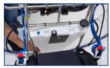
7) Slide the tank under the engine, through the airframe and then push down to locate the bottom lugs onto the frame
