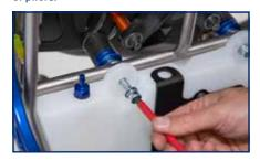
**4)** Using the 6mm allen key, remove the bottom engine mount bolts that secure the tank in place
