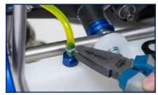
**3)** Using the pliers, carefully remove the fuel pipe by pinching the clip and sliding it upwards along the pipe
