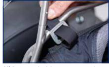
**11)** Reconnect both harness straps to the top of the Maverick airframe using the opposite sequence from removal
