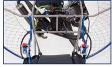
**6)** Carefully lift the engine away from the airframe to allow the Extended Range tank to be inserted into place
