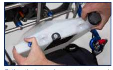
5) Slide the fuel tank upwards and towards the harness to remove it from the Maverick airframe
