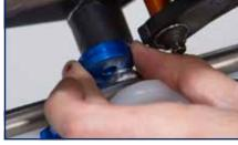
8) Push the top of the tank towards the airframe to align with the engine mounts, ensuinge the 4 x 5mm spacers are in place
