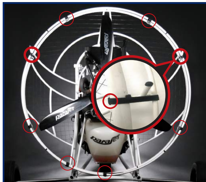
1 Strap & ladder lock buckle used for additional outer-ring installation
