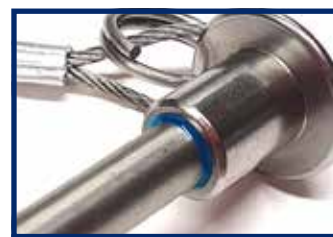
2 Apply thread locking liquid
