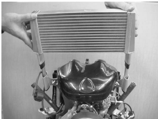
Picture 2. The fitting the radiator in the correct orientation.
