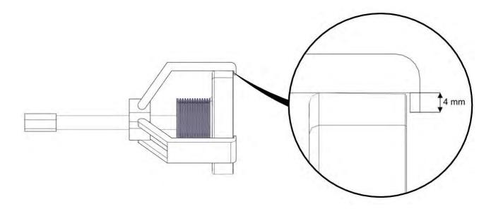
Position the extractor (10) on the clutch bell (9).
