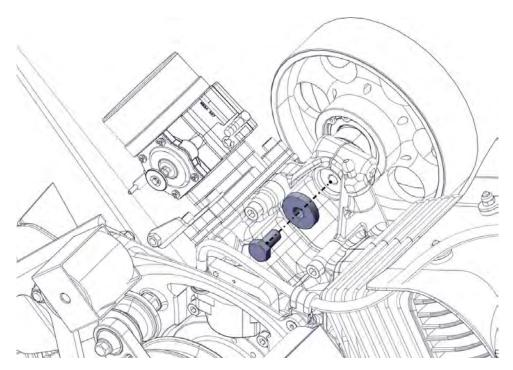
Remove the Allen screw M6x35 on the eccentric side.
