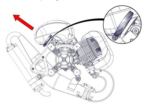
Fold the sleeve inwards and remove it from the airbox. Remove the Snaplock.
