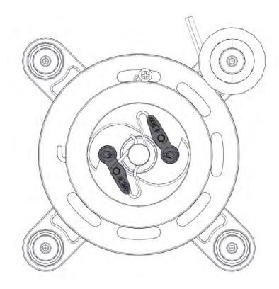
Insert the 4 flange head screws M6x63 (1) with threadlocker (Loxeal 24-18/Loctite 222 recommended) into the manual starter bracket (2).
