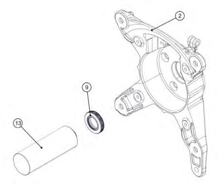
Carefully add silicone paste (Three Bond 1215) to the crankcase profile as shown in the figure. Height, width silicone profile:  $2 \text{ mm} \times 2.5 \text{ mm}$ .
