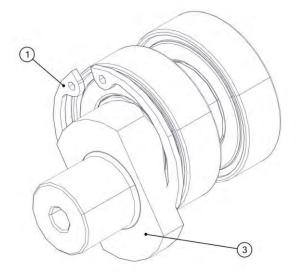
Heat the central part of the pulley to 120 °C. Insert the eccentric (3) with the 2 bearings in the pulley (2).
