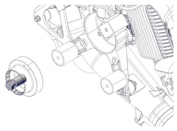
Remove the 2 Allen screws M5x20 (1) with washers (2) from the coil (3). Remove the coil (3).
