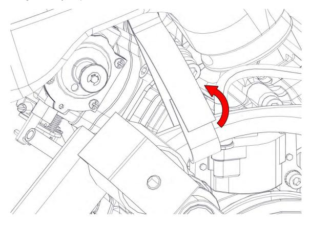
Loosen the screw of the clamp securing the sleeve to the carburettor and remove the airbox.
