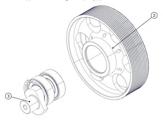
Position the Seeger ring (1) in the seat inside the pulley (2).
