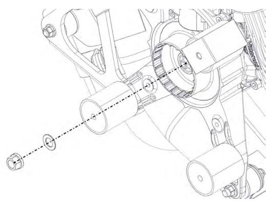
Screw the flywheel extractor into the starter cup.
