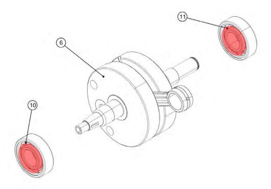
Heat the transmission side crankcase to 120  $^{\circ}$ C. Insert the crankshaft (6) with the bearings.
