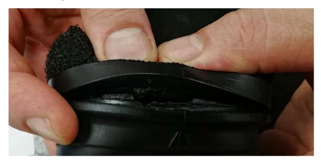
Check the filter, in particular the bonding with the sleeve and the various parts of the sponge.
