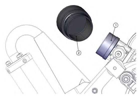
Check the integrity of the airbox. Check the sleeve groove.
