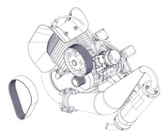
Insert the hexagonal screw M8x16 with washer into the eccentric of the pulley.
