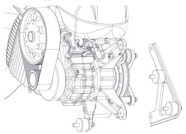
Remove the 2 remaining engine rubber mountings.
