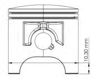
Measure the diameter of the cylinder 10 mm from the top.
