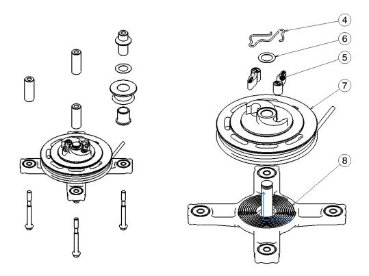
Remove the rope by untying the knot and pulling it off the pulley
