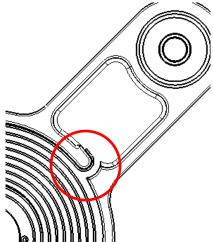
Insert the spring of the hooks on the central pin and turn it, if any blockage or jamming occurs the pin and structure must be replaced.
