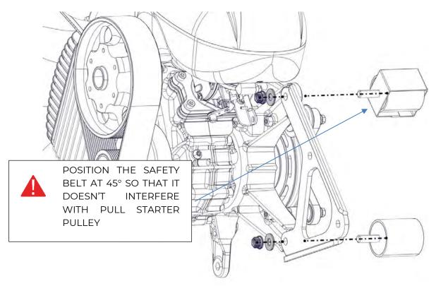
Insert the 2 remaining engine rubber mountings and tighten by hand.
