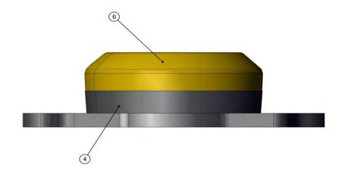
Clean the bushing and cylinder from gasket residue.
