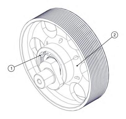
Heat the central part of the pulley to 120 °C. Remove the eccentric (3) with the 2 bearings from the pulley (2).
