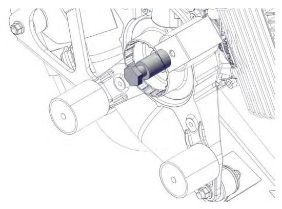
Turn the central pin of the extractor until the flywheel is removed from the crankshaft.
