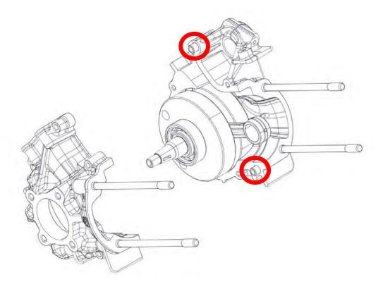
Add Wurth paste 0893921501 to the screws M8x16. Insert the 5 Allen screws M6x35 (3), the 2 Allen screws M6x40 (4) and tighten with the torque shown in the figure.
