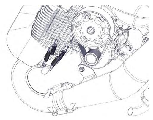
Remove the 3 self-locking nuts M8 with washers.
