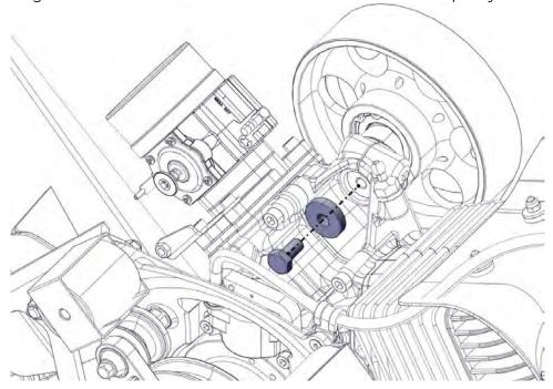
Add Wurth paste 0893921502 to the screw M6x35. Insert the Allen screw M6x35 on the side of the eccentric.
