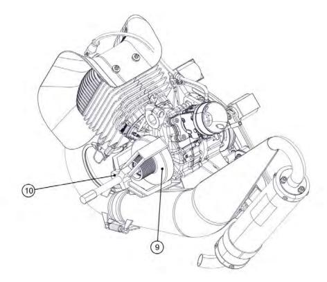
Turn the central pin (11) until the clutch bell (9) is removed.
