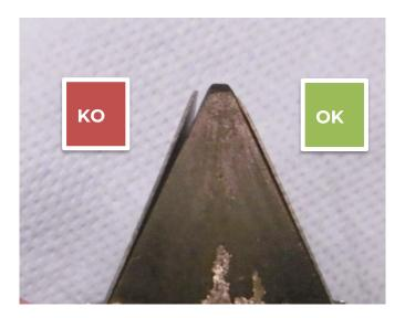
If the previous checks are not passed or if routine maintenance is required, replace the petals.
