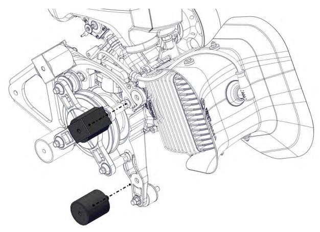
Remove 3 self-locking nuts M8 and 3 rubber mountings of the exhaust system.
