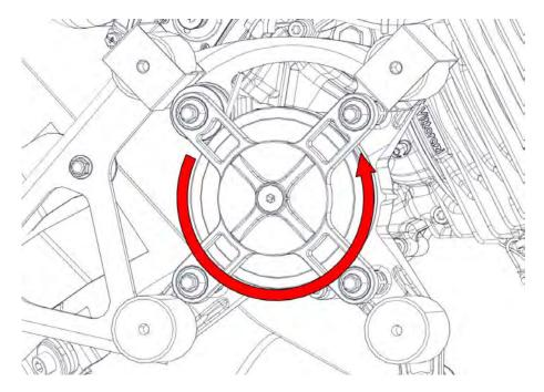
Gradually unscrew the 4 flange head screws M6x63 (1) on the manual starter bracket (2). Follow the sequence highlighted by the blue arrows. Maximum two complete turns per screw. After removing the manual starter, the cup (3) mounted on the flywheel is visible.
