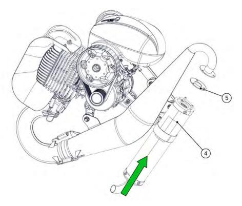
Insert the 3 nuts on the silencer then the 3 self-locking nuts. Tighten up to 10 Nm. Tighten the first 3 nuts progressively to guarantee a correct alignment of the silencer
