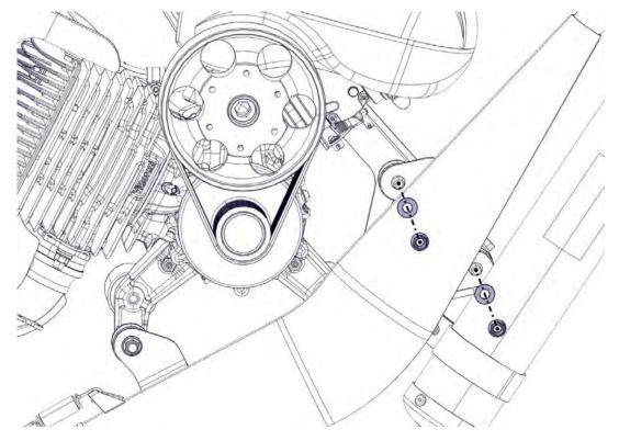
Hook in the 4 bushing springs. Run a cable around the four bushing springs, insert a clamp on the ends and tighten with pliers. (Check chapter 3.7 for spring assembling operations)
