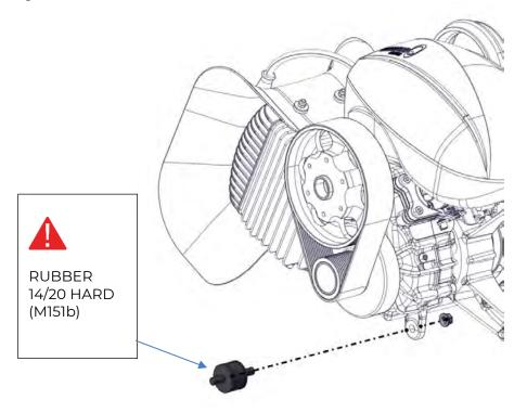
Insert the 2 exhaust system rubber mounting shown in the figure, the 2 self-locking nuts M8 and tighten to 15 Nm.
