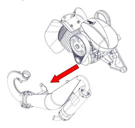
Remove the 2 self-locking nuts M8 with washers and the 2 rubber mountings from the motor mount.
