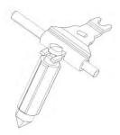
Check the condition of the diaphragms: they must be soft and free of cuts, otherwise they must be replaced. For routine maintenance, follow the table.
