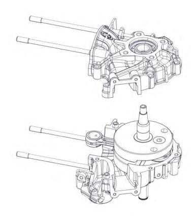
Remove the oil seal (9) from the crankcase support (2) on the side shown in the figure.
