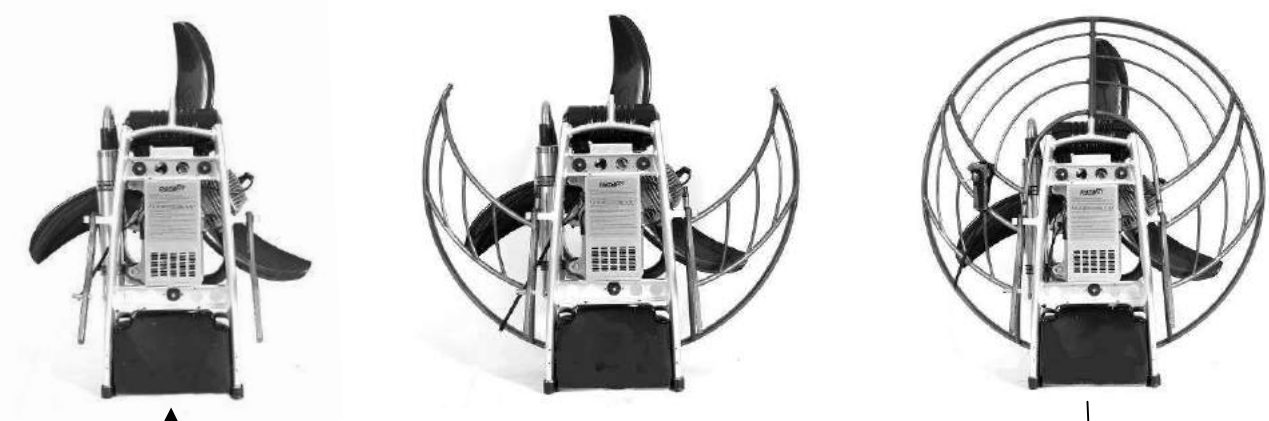
Left: Internal guard vertical support slots through chassis holder before lower connectors are locked in position
