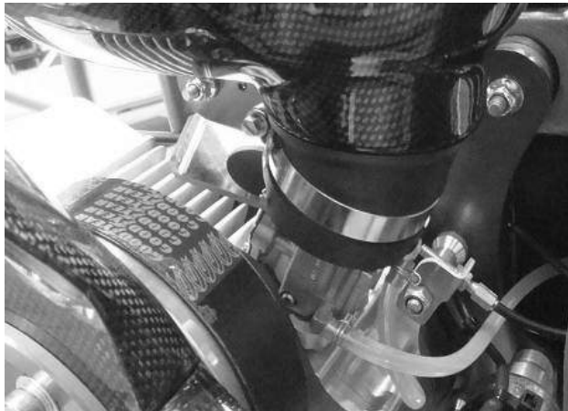
Choke valve shown in "ON" position. Use this position to prime and start the engine initially
