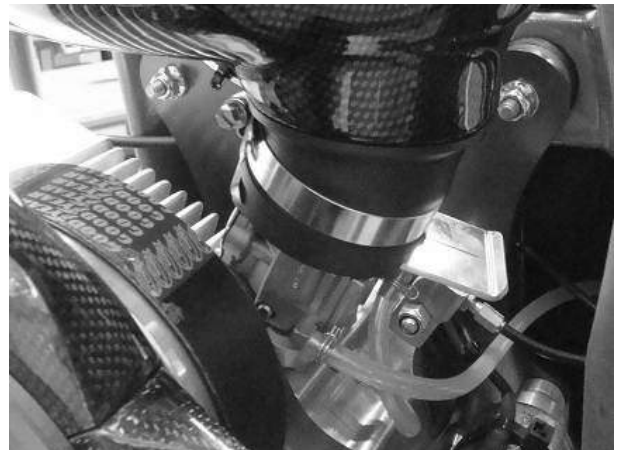
Choke valve shown in "RUN" position. Use this position to run the engine for flying
