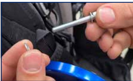
4) Remove one of the metal washers, retaining one washer on the head side of the bolt.
