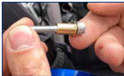
5) Locate the brass bush onto the bolt ensuring the bush collar is orientated towards the head of the bolt.
