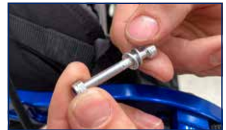
3) Turning it by hand, remove the hex nut from the end of the bolt provided in an anti-clockwise direct.
