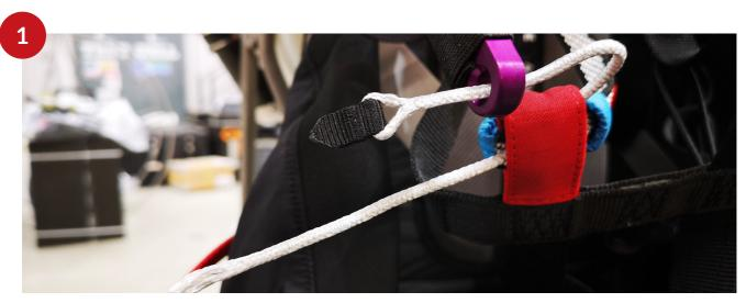
Firstly, untie the soft link in its current configuration. Once untied, position the tab end of the soft link (webbing end) on the outside of the harness arm. Pass the free end through the harness arm, then route it back through the harness webbing.
